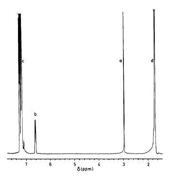
Figure 5 <sup>1</sup>H n.m.r. spectrum of  $\alpha, \omega$ -N,N'-dimethylamino PC ( $\overline{M}_n = 2500$ )
