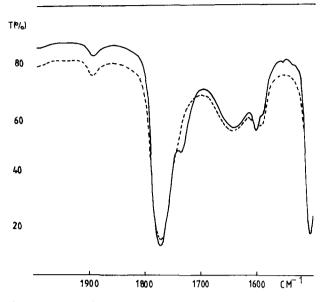
**Figure 2** Comparison of the i.r. spectra of PC prepared in the presence  $(--, \overline{M}_n = 8200)$  and absence  $(--, \overline{M}_n = 7200)$  of HBA
