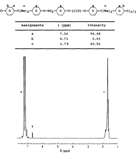
Figure 4 <sup>1</sup>H n.m.r. spectrum of a PC sample prepared in the presence of HBSA as a chain stopper ( $\overline{M}_{p} = 7500$ )
