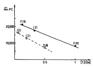
Figure 1 Dependence of the number-average molecular weight (as determined by size exclusion chromatography using polystyrene calibration) on the HBA/bisphenol-A molar ratio ( $\bigcirc$ ) and the HBSA/bisphenol-A molar ratio ( $\square$ ). The polydispersity is given in parentheses
