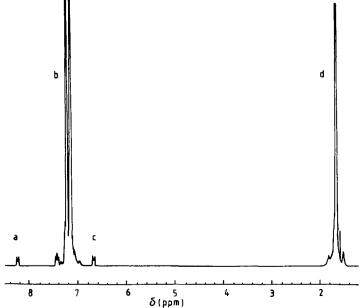
Figure 3 <sup>1</sup>H n.m.r. spectrum of a PC sample prepared in the presence of HBA as a chain terminator ( $\overline{M}_n \approx 18\,000$ )
